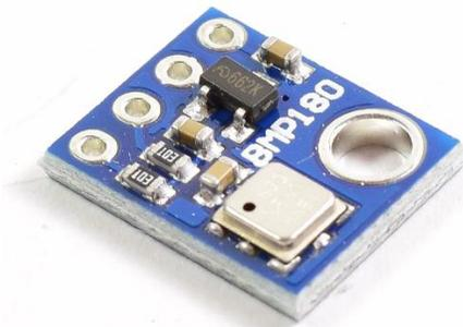
Figura 21 Sensor BMP180 (Fuente: [https://media.naylampmechatronics.com/664-superlarge\\_default/sensor-de-presion-bmp180.jpg](https://media.naylampmechatronics.com/664-superlarge_default/sensor-de-presion-bmp180.jpg))
