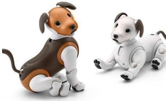
**Figura 2.8** Robot AIBO
