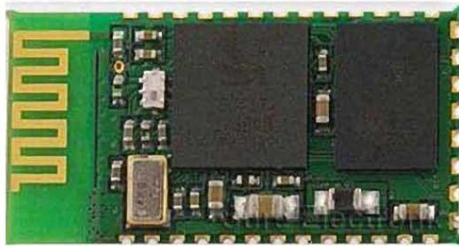
Figura II, 8 Modulo Conversor Bluetooth a Serial
