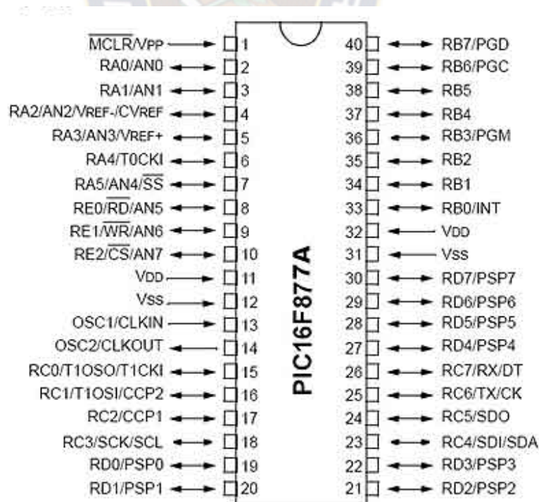
Fig.5 Diagrama de pines del PIC16F877A
