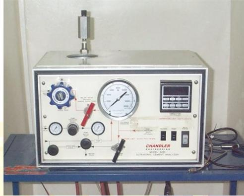
*Fig g-1 Ultrasonic Cement Analyzer (UCA)
