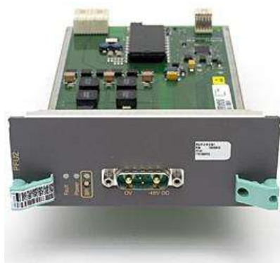
Figura 3.7: Power Filter Unit 2 (PFU2).
