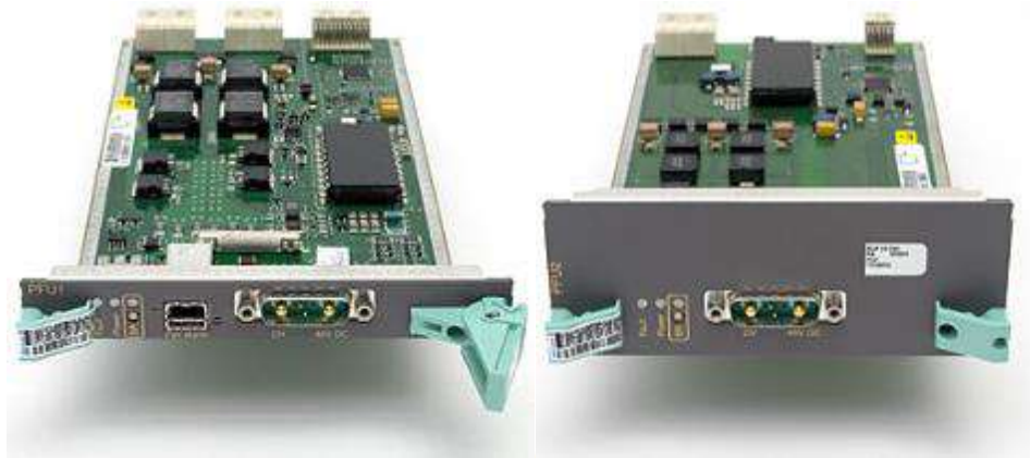
Figura 3.12: Power Filter Unit (PFU).
