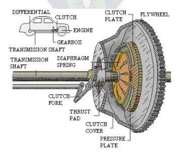
The clutch of a car consists of two plates; one connected to the engine crankshaft, and the other to the gearbox. A diaphragm spring holds the plates together, so that friction transmits the rotation of the crankshaft to the gearbox. When you press the clutch pedal, the spring flips backward, and the plates separate, enabling you to select a different gear.
