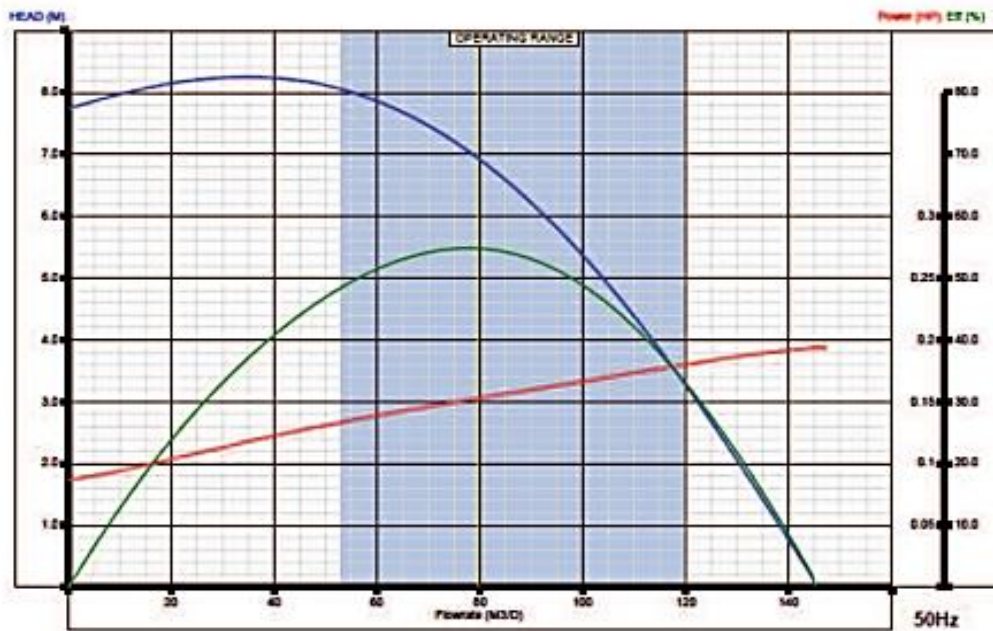
P6 Pump 400 SERIES 1 Stage Performance Curve RPM=2917 Sp.Gr.=1.0
