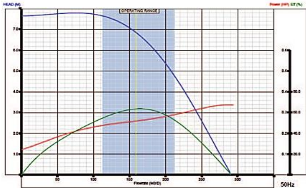
P12 Pump 400 SERIES 1 Stage Performance Curve RPM=2917 Sp.Gr.=1.0
