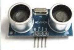
A blue HC-SR04 ultrasonic distance sensor with two circular transducers and a three-pin header.                                       | 4.5V-10 mA<br>5V- 15 mA |
