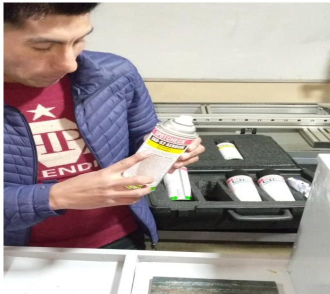
Fig. 3.22. Revelador SPROTCHECK SKD-S2 aerosol ASTM E-1417, ASTM E-165,
