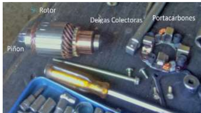
Figura 68. Rotor y portacarbonos (Toyota Land Cruiser)
