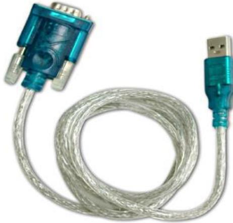
**Figura 3.10 conversor usb- serial**
