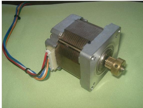
**Figura 4.10 Motor paso a paso**
